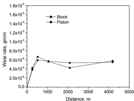
Fig. 3 Variation of wear rate (gm/m) with the variation of sliding distance (m) at applied pressure of 0.30 MPa (Load 5N) and sliding velocity 0.29 ms<sup>-1</sup>
