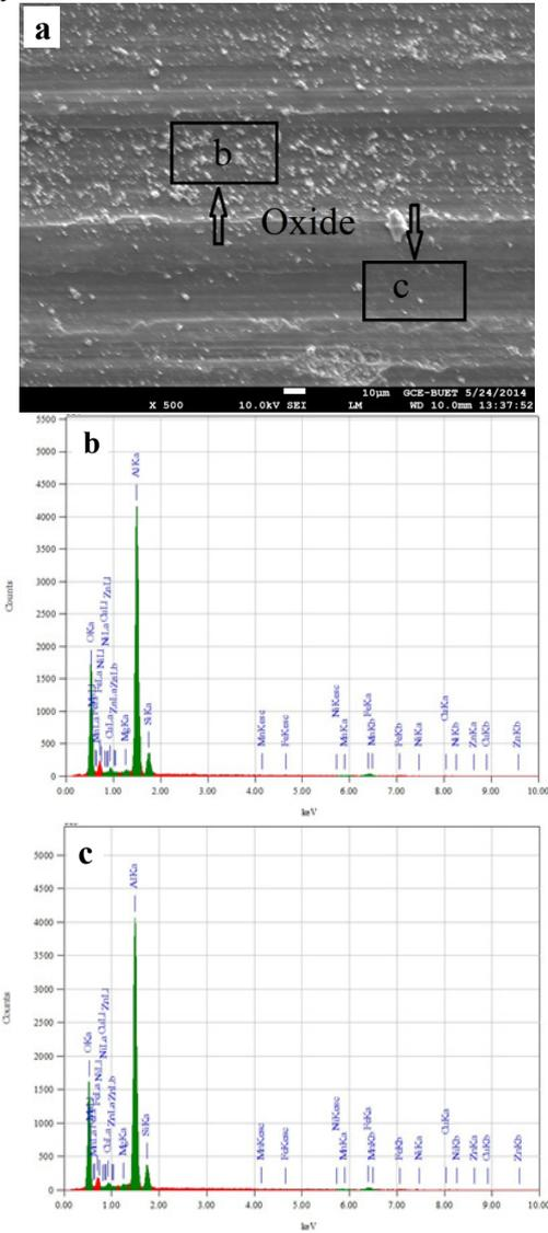
Fig. 9 SEM images of worn surfaces of aluminium engine piston after wear at 1.4 MPa applied pressure and sliding distance of 4200m
